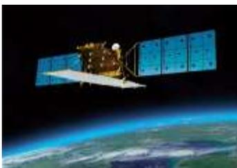
The state-of-the-art L-band Synthetic Aperture Radar-2 (PALSAR-2) aboard ALOS-2, which is active microwave radar using the 1.2GHz frequency range, will, in responding to society's needs, have enhanced performance compared to the DAICHI/PALSAR. The PALSAR-2 can observe day and night around the clock.
