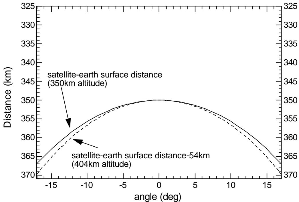
Figure 1. Satellite to Earth surface distance in the cases of 350km and 404km satellite altitudes.
