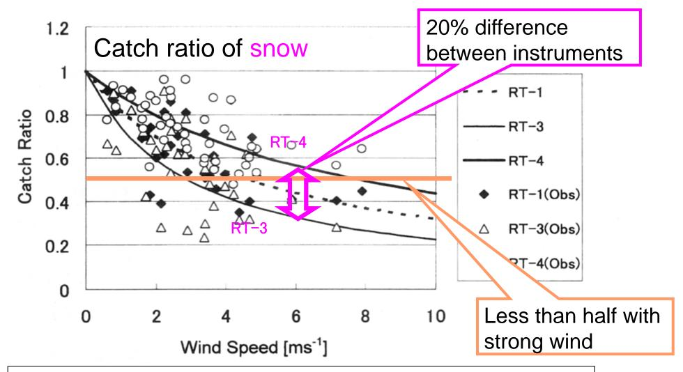
Catch ratio of snowfall and wind speed with 3 types of JMA rain gauges. Dots show observation results from each gauges, and curves show regression curves from them.
