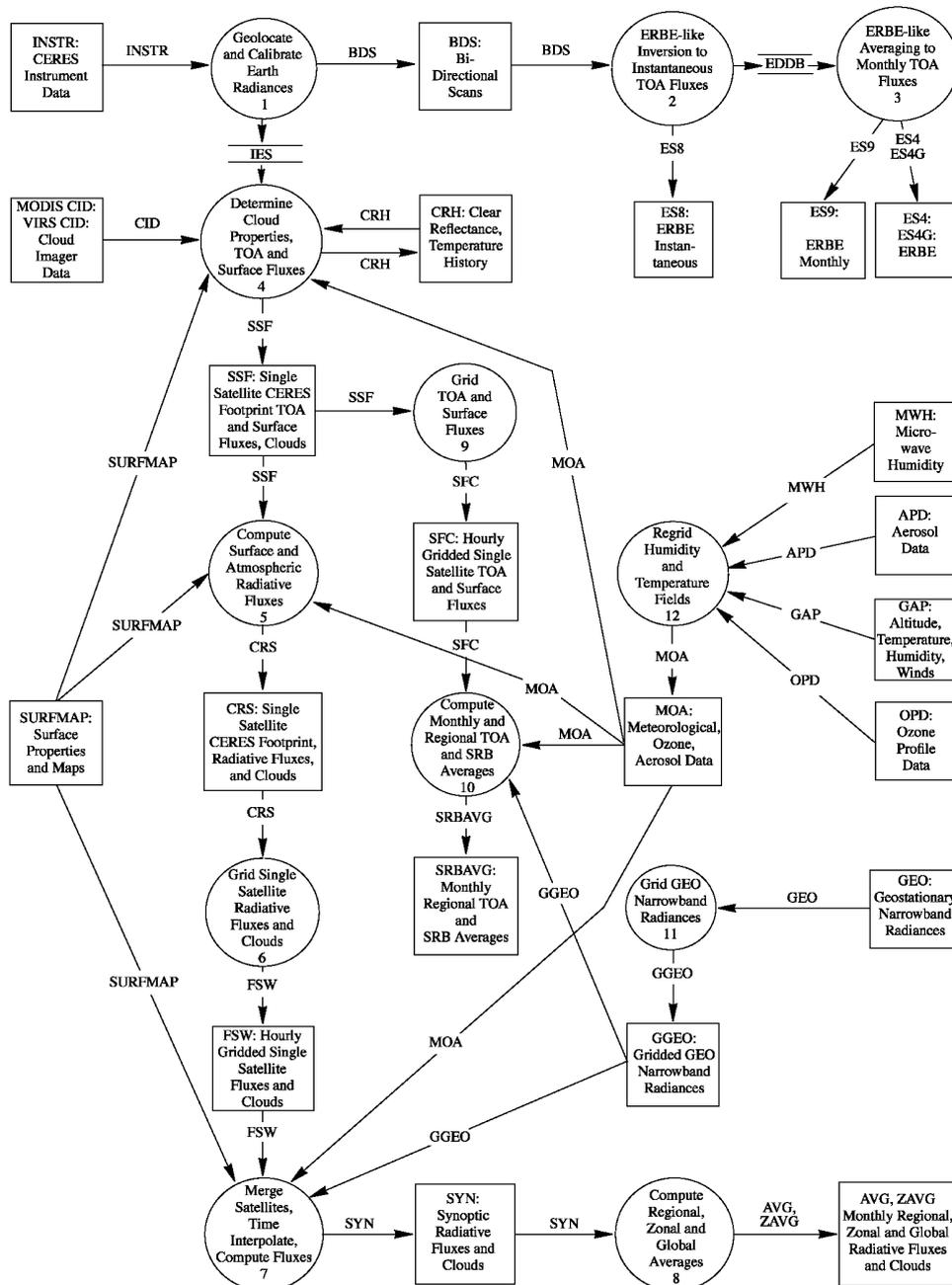
Figure 4.1-10 CERES DATA FLOW DIAGRAM
