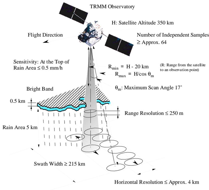
Figure 2.6-3 Measurement Concept of Precipitation Radar on board TRMM
