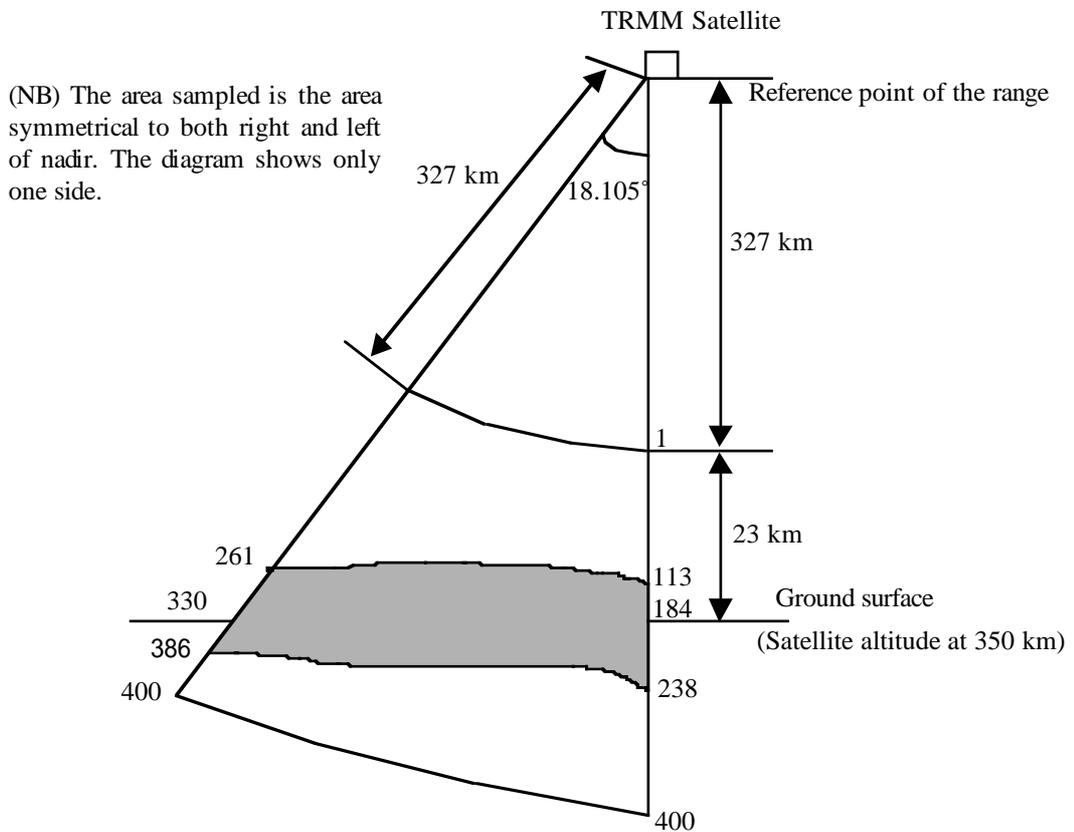
Figure 2.6-11 Data Sampling during External Calibration Mode
