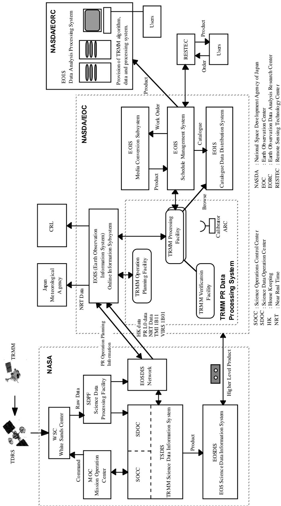
Figure 3.2-1 Relationship between the TRMM PR Data Processing System and Foreign Organizations
