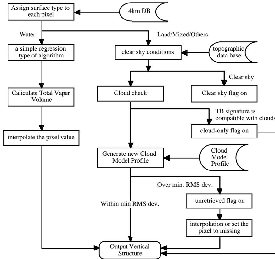
Figure 4.1-9 TMI Level 2A-12 Process Flow Diagram
