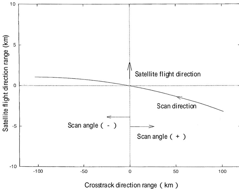
Figure 2.6-13 Scan Track of PR
