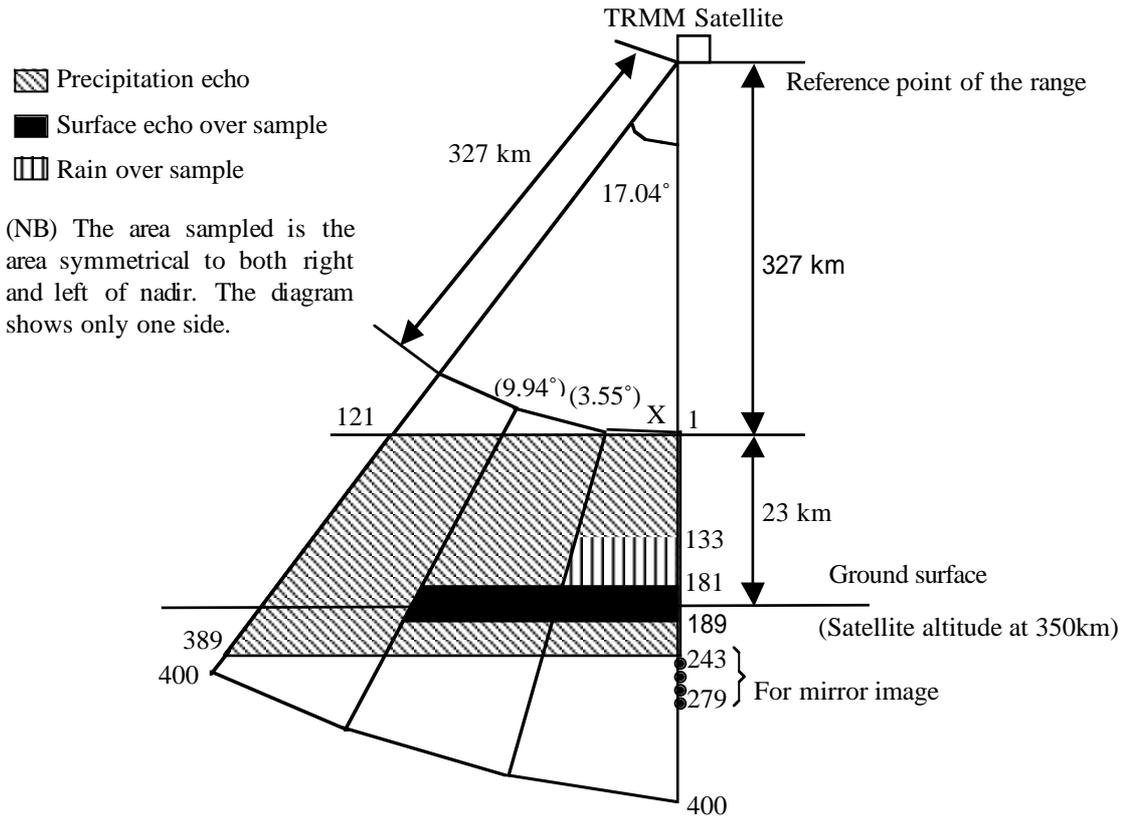
Figure 2.6-10 Data Sampling Area during the Observation Mode
