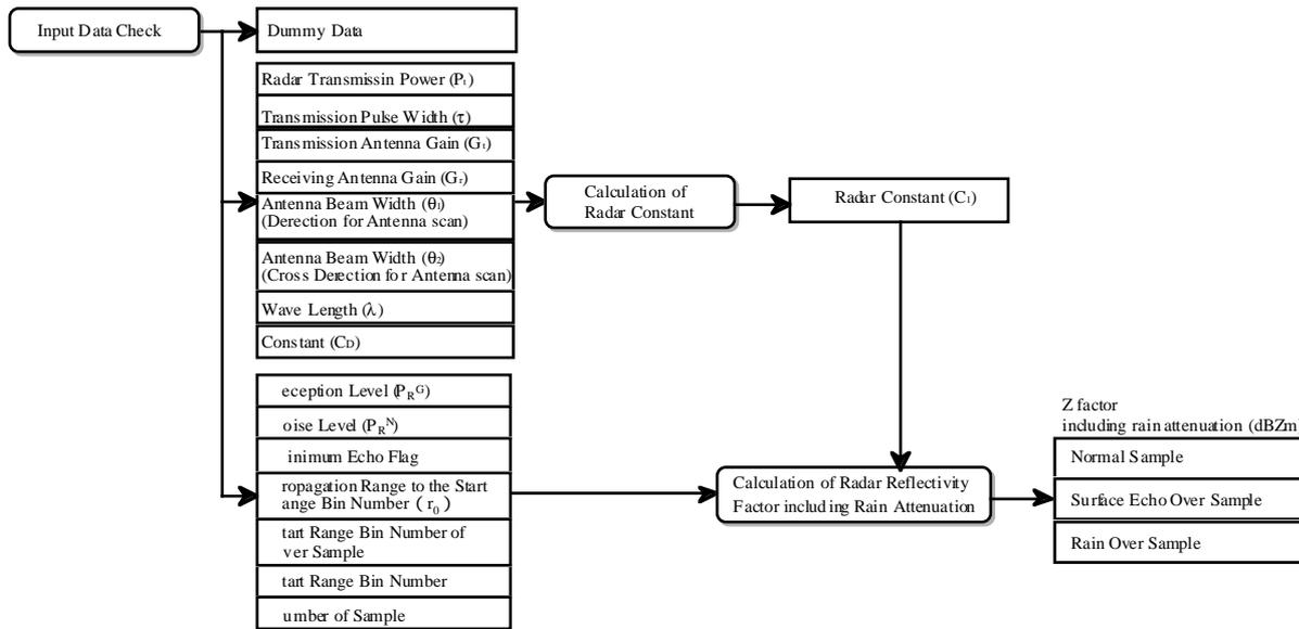
Figure 4.1-8 Relationship between functions of 1C21 processing
