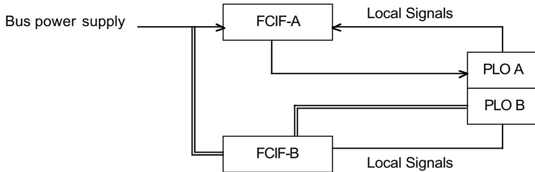
Figure 2.6-8 Operation of PLO when FCIF-A System is turned on
