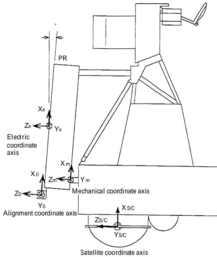
Figure 2.6-12 Coordinates Axes of the Satellite and PR
