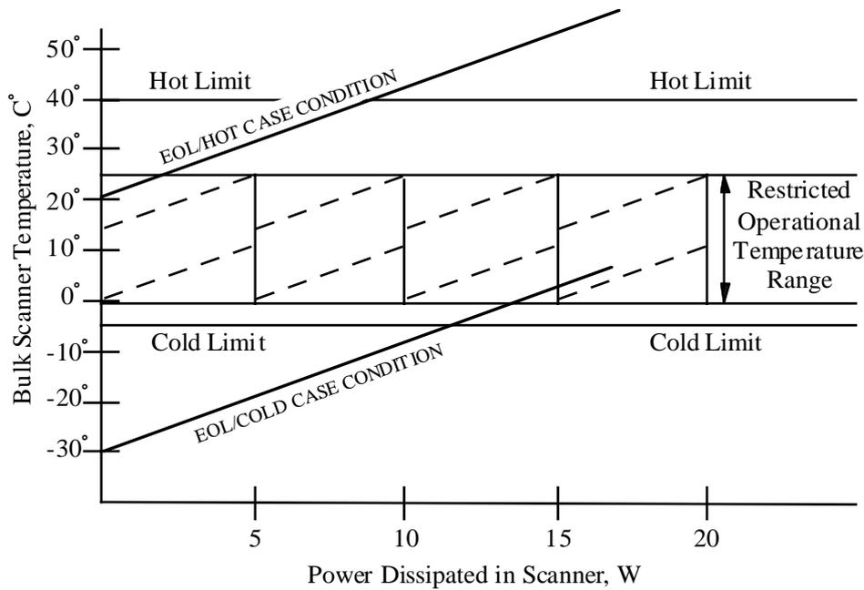
Figure 2.5-4 Thermal Monitoring
