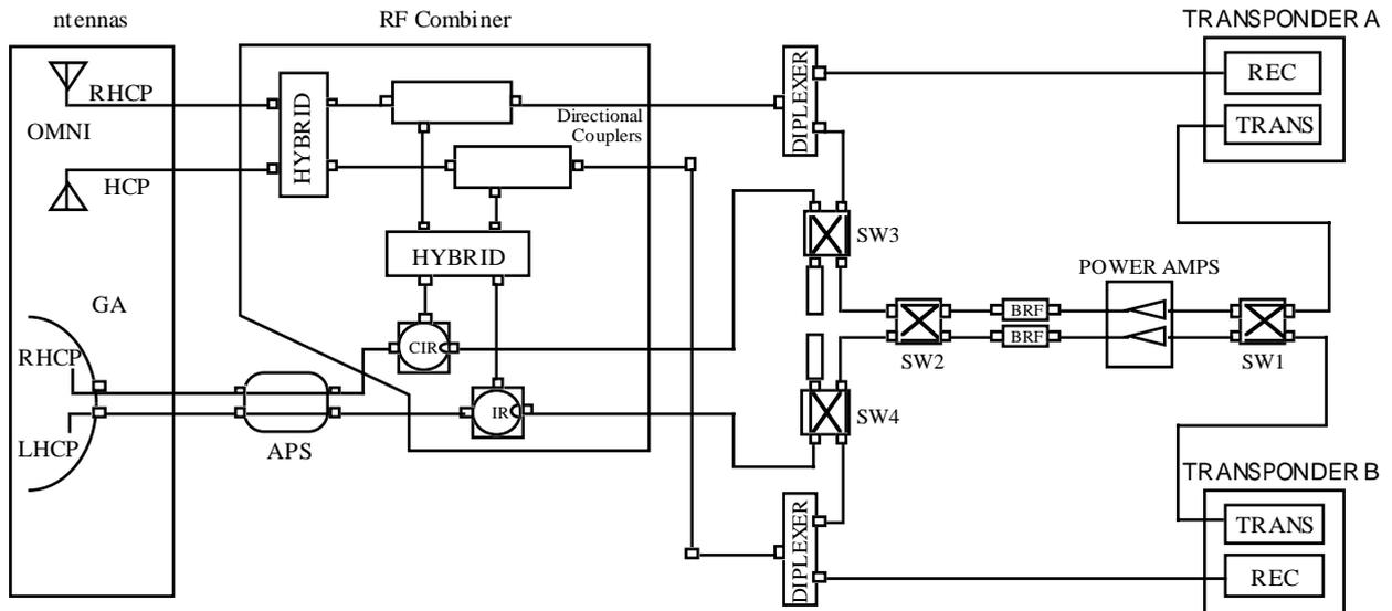
Figure 2.1-6 RF Communications Subsystem Block Diagram
