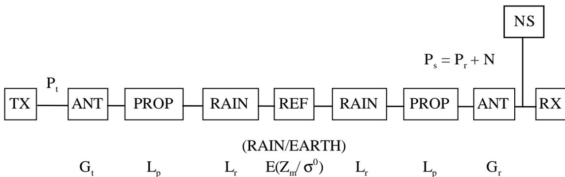
(NOTE) TX: Transmitter, ANT: Antenna, PROP: Propagation, REF: Reflection, NS: Various Noise Sources, RX: Receiver
