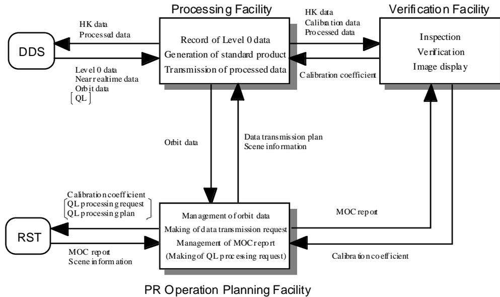
Figure 3.2-4 Operation Configuration (Observation mode)
