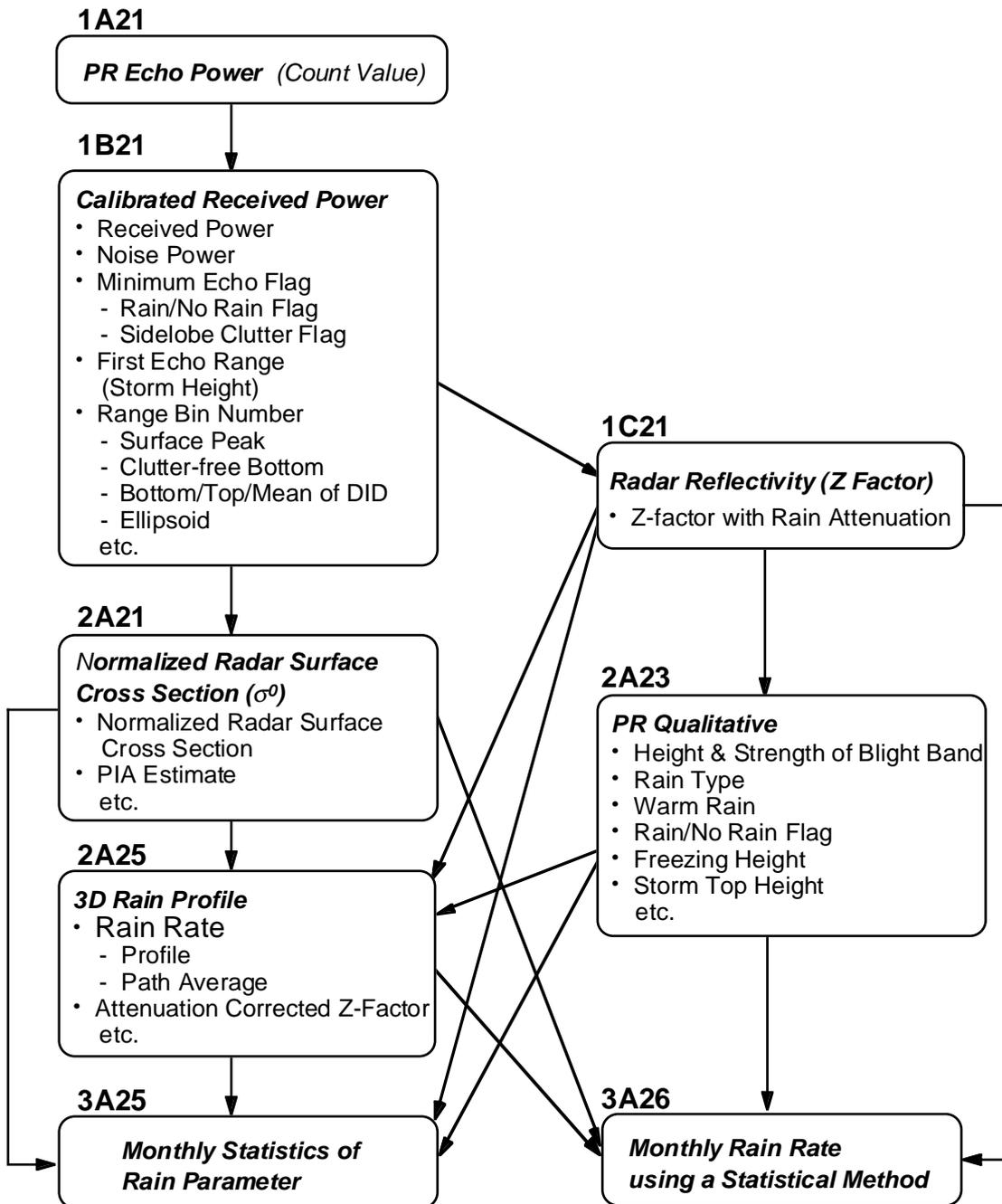
Figure 4.1-2 Overall flow chart of precipitation radar algorithm
