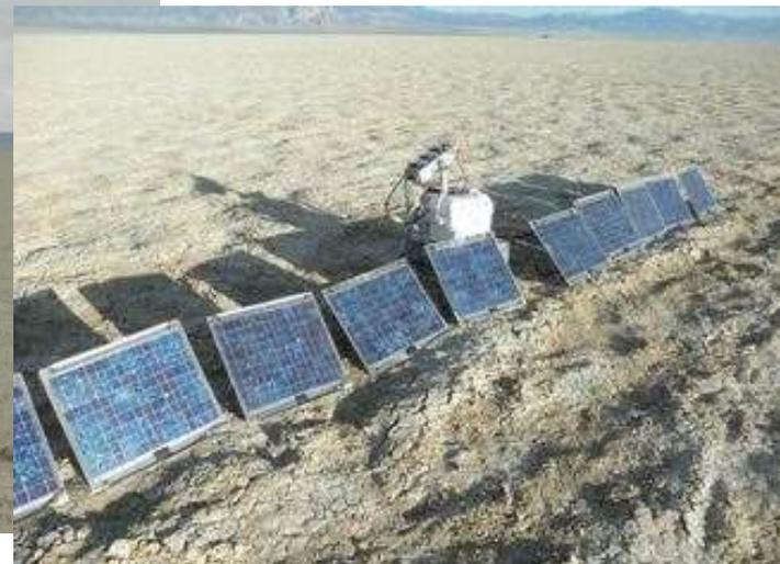
Portable Apparatus for Rapid Acquisition of Bidirectional Observation of the Land and Atmosphere
