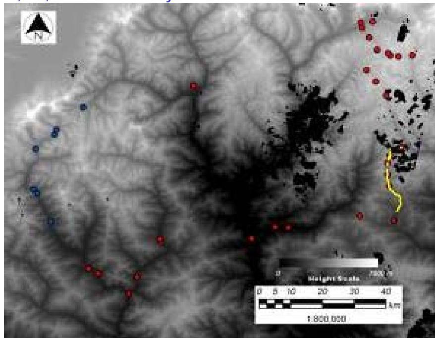
Magnified PRISM DSM mosaic and location of GPS measurements points (yellow: continuous measurement in 2010; red: CPs in 2010; and blue: CPs in 2011).
