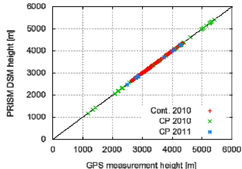
Comparison of height between the GPS measurements and PRISM DSM (red: continuous measurement in 2010; green: CPs in 2010; and blue: CPs in 2011).
