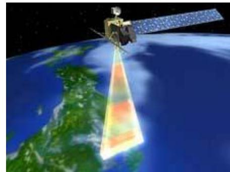
AVNIR-2 can observe with **10m resolution in 70km swath**, and it can be changed the observation area by **pointing capability**
