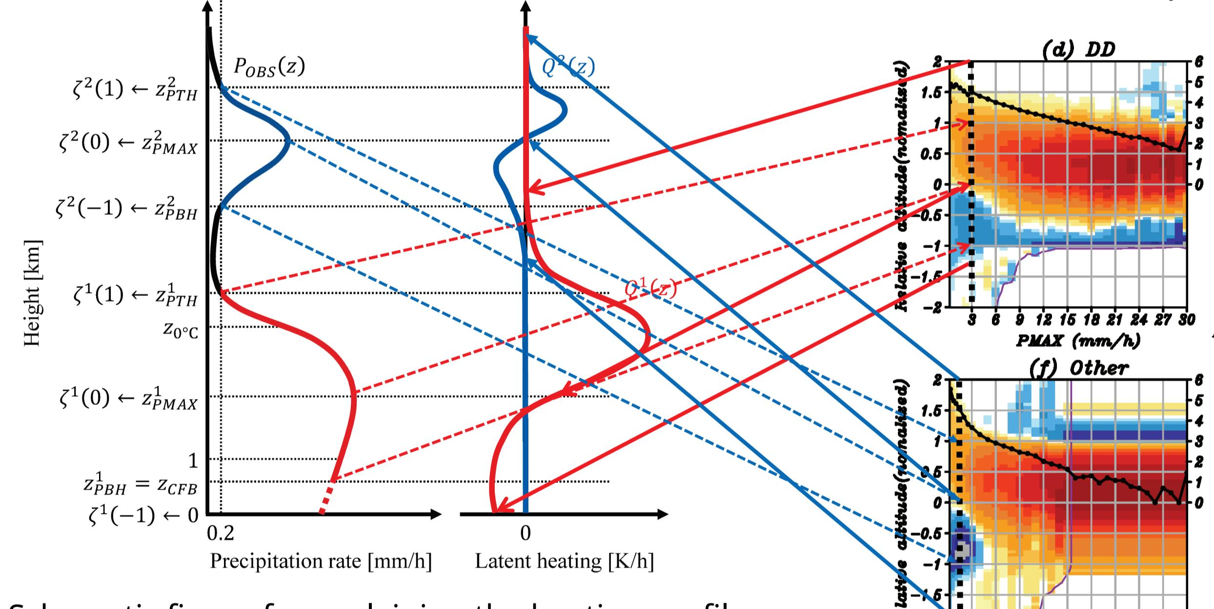
Schematic figure for explaining the heating profile retrieval using the PMX method
