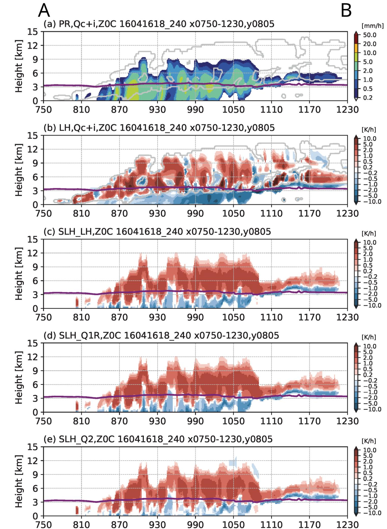
LFM-simulated prec and heating vs. SLH estimates using GPM prec
