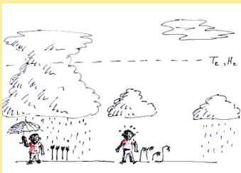
Figure 2. The TAMSAT algorithm. Comparison with local gauge data is used to derive threshold temperature T_c , which identifies rainy cloud.
