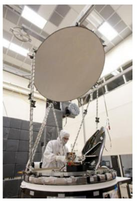
Figure 1.2-2 GPM Microwave Imager (GMI) Provided by NASA
