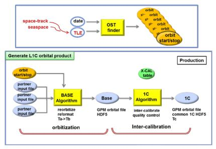
Figure 3.5-2 L1C Processing Flow Standard Production
