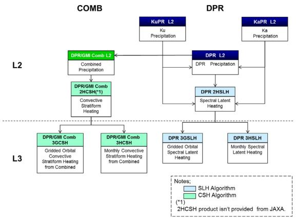
Figure 1.5-1b GPM Product Processing Flow ( Downstream of Figure 1.5-1a)
