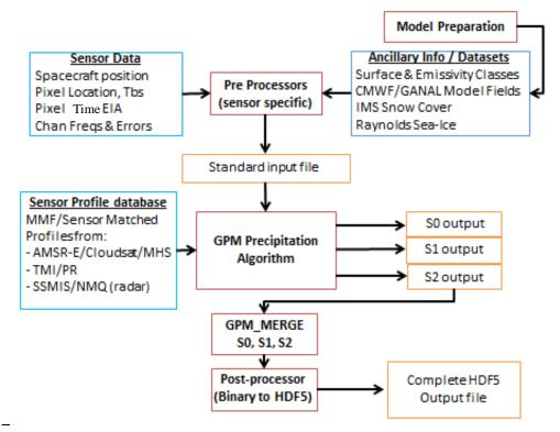
Figure 3.5-4 Overview of the Processing Steps for the GPM Precipitation Algorithm
