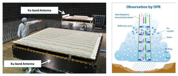
Figure 1.2-1 Dual-frequency Precipitation Radar (DPR) of Ku-band Sensitive to Strong Rain and Ka-band Sensitive to Light Rain and Snow
