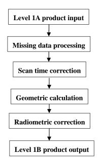
Figure 2.5-1 DPR Level 1B Standard Processing Flow
