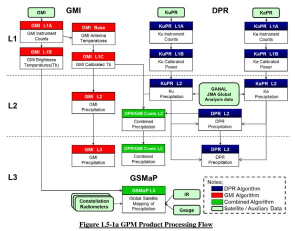
1.5.1 GPM Processing Flow
