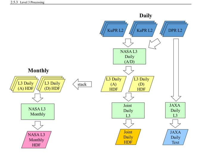
Figure 2.5-3 Flow of the L3 Standard Processing Algorithm
