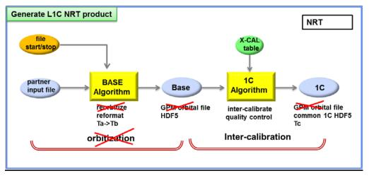
Figure 3.5-3 L1C Processing Flow Near-Real-Time
