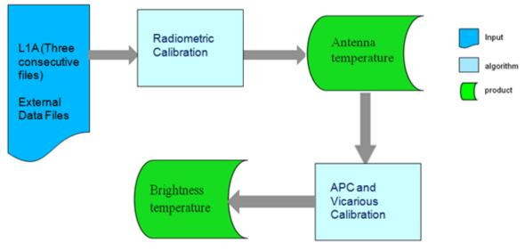
Figure 3.5-1 The Top-level Flow Chart of the GMI L1B Algorithm
