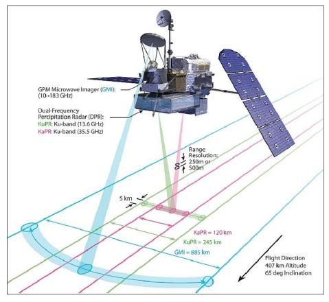
Figure 3.2-1 Schematic View of the Observation Geometries With the GPM Core Instruments (Image Credit: NASA)
