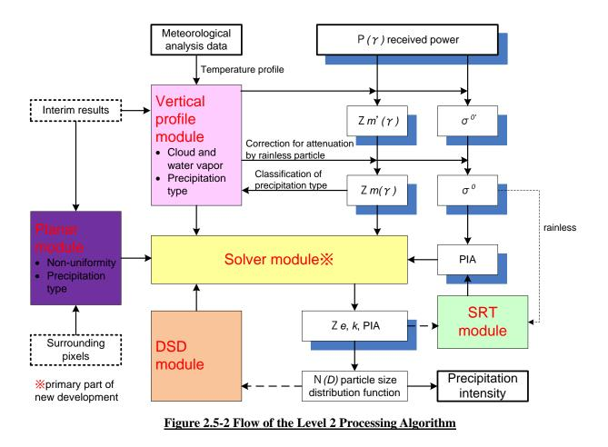
DSD: Drop Size Distribution, SRT: Surface Reference Technique, PIA: Path Integrated Attenuation
