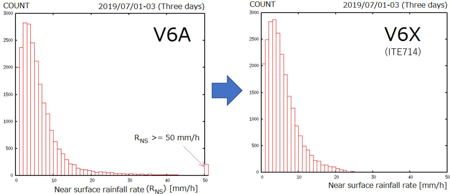
The V6A problem of large near surface rainfall rate ( $N_{RS}$ ) for the re-classified stratiform type by the Slope method is solved by introducing an external filter in the CSF module. The threshold TH introduced in V6X is
