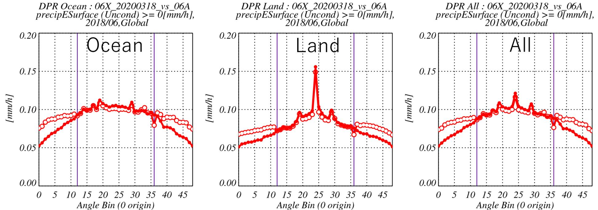
Differences between V06A and V06X in the Dual-frequency product were found in the outer swath.
