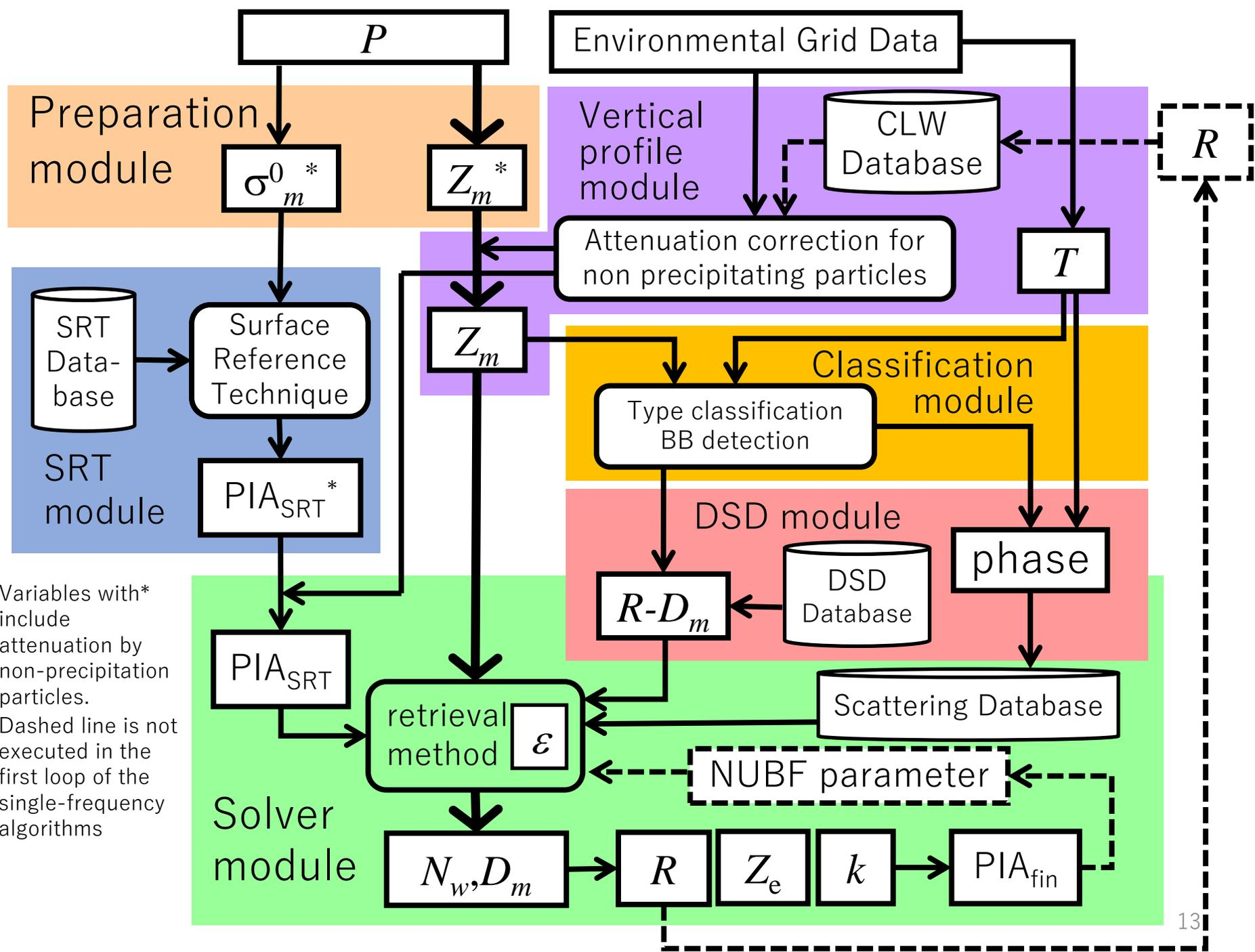
Variables with\* include attenuation by non-precipitation particles. Dashed line is not executed in the first loop of the single-frequency algorithms
