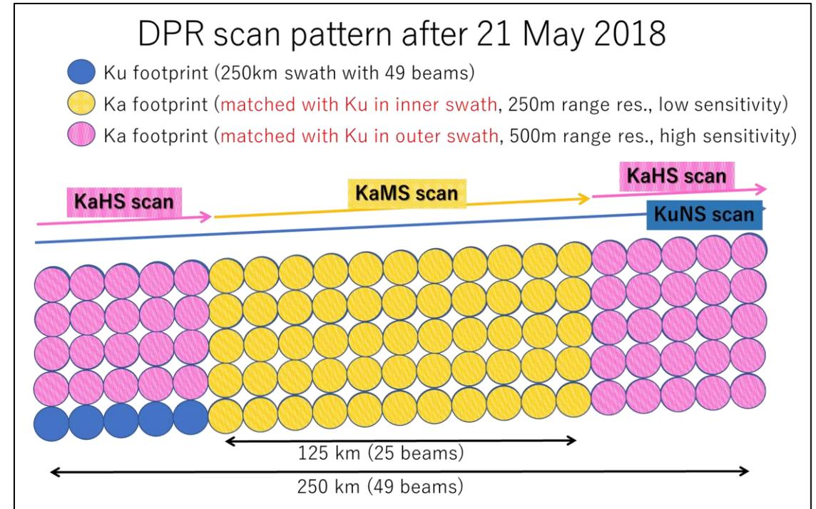
The full-swath coverage after the DPR scan pattern change provides consistent dual-frequency computations across the full swath. To realize it, we need to develop L2 algorithms to correspond to the new scan pattern.
