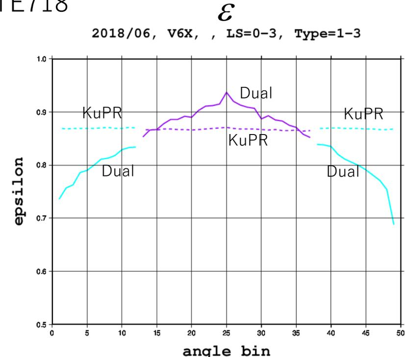
While  $\varepsilon$  is almost constant in KuPR algorithm,  $\varepsilon$  decreases at larger incident angle in Dual-frequency algorithm.
