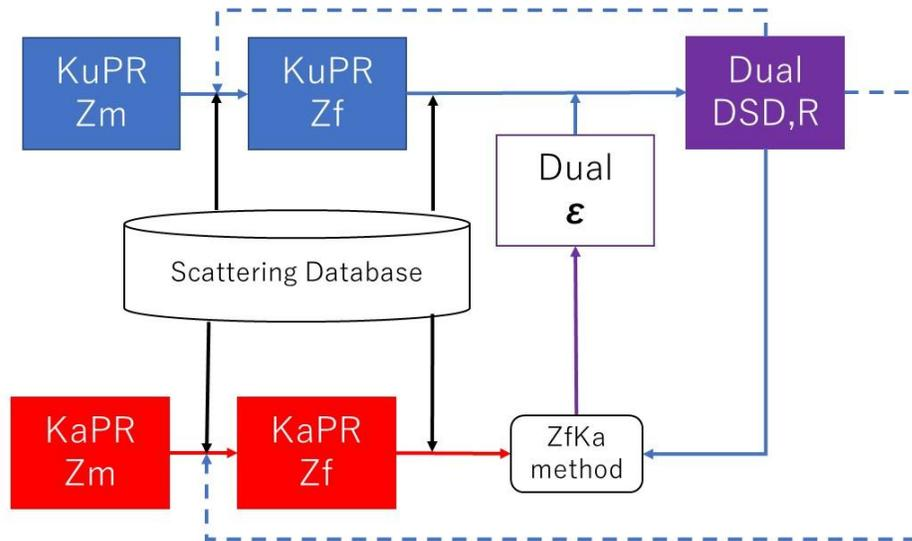
" $\varepsilon$ " is an adjustment factor in the relationship between precipitation rate  $R$  and volume-weighted mean drop size  $D_m$  (so-called,  $R$ - $D_m$  relationship).
