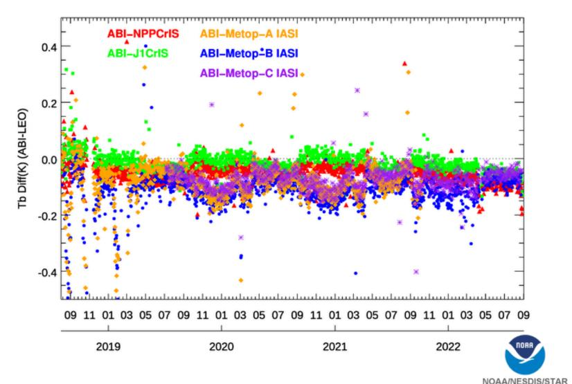
NOAA uses GSICS intercalibration methods to track the performance of the GOES ABI instruments. The figure to the left shows brightness temperature biases from daily matchup statistics for the 9.6 µm channel against five reference instrument, the S-NPP and NOAA-20 Cross-track Infrared Sounders (CrIS) and Metop-A, -B, and -C Infrared **Atmospheric Sounding** Interferometers (IASI). The bias are consistent at the 0.2 K level and show improved behavior over time.
