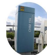
Low power lidar and ceilometer
