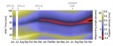
The CPR antenna mispointing trends suggest that all Doppler velocity measurements prior to December 2024 were influenced by an extra source of bias, affecting not only low echo-level values but also the entire range, including the surface return (which typically exceeds 30 dBZ)
