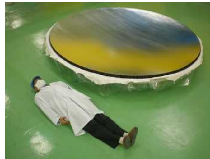
Full size (2.5m dia.) CPR Antenna BBM with high surface accuracy
