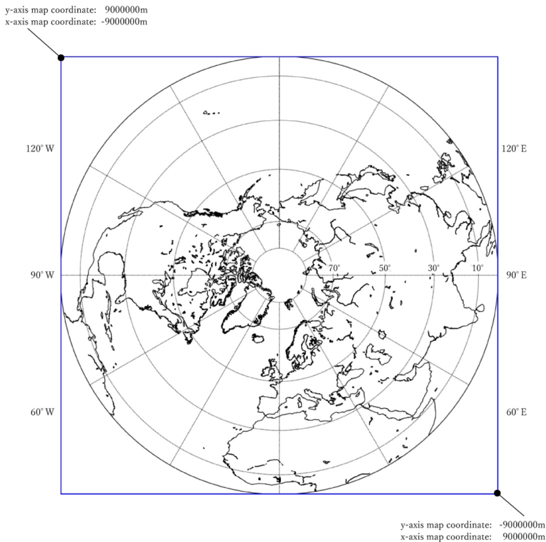
Figure 3.4-6 EASE-Grid 2.0 Projection Definition (Northern Hemisphere, Lambert Azimuthal)
