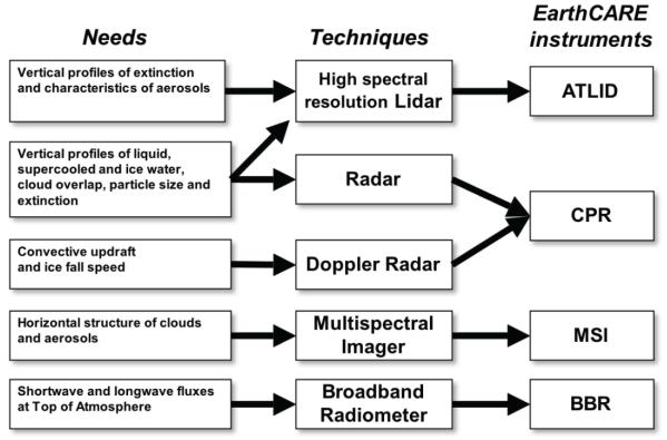
Figure 1 Relationship between target geophysical parameters and instruments
