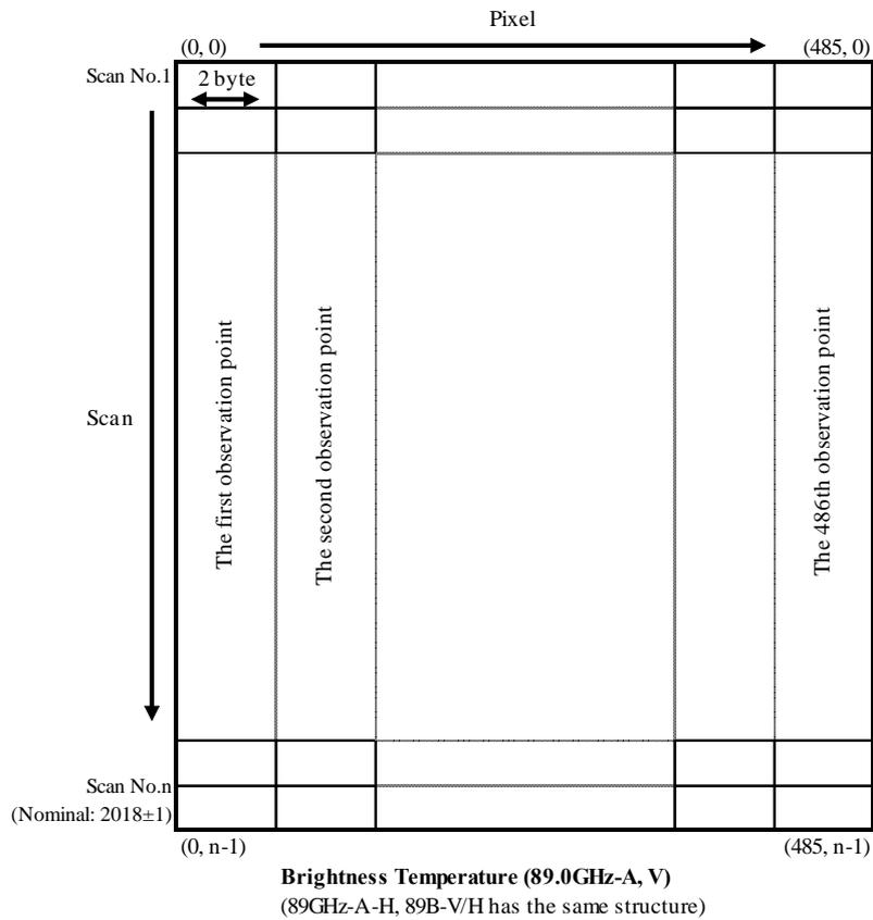
Figure 3-3 Structure of Brightness Temperature
