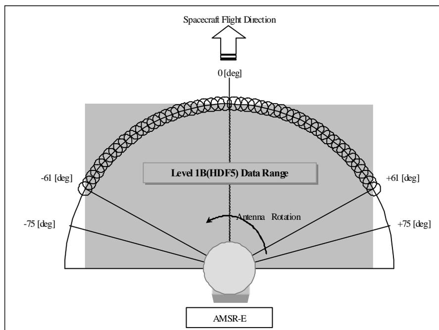
Figure 3-1 the data range of one scan for AMSR-E Level1B(HDF5)
