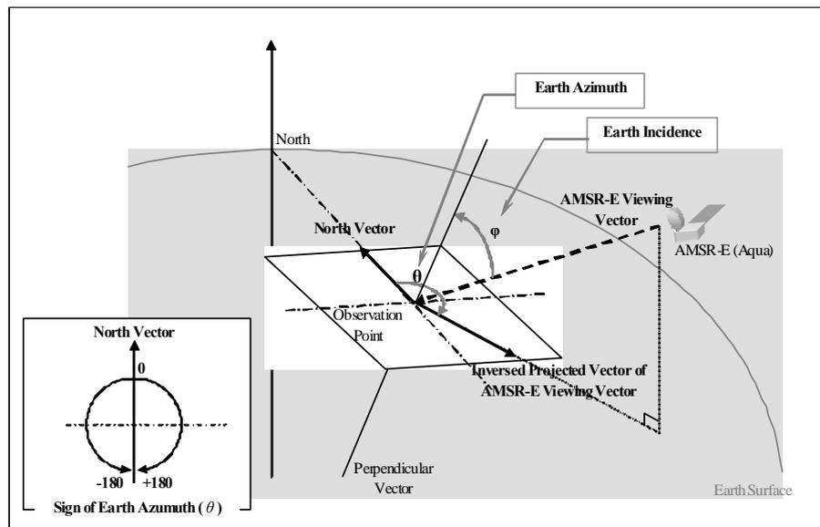
Figure 4-3 The definition of Earth Azimuth and Incidence
