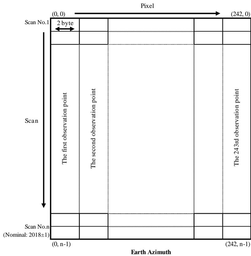
Figure 3-9 Structure of Earth Incidence / Earth Azimuth
