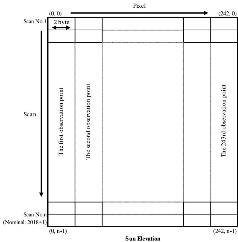
Figure 3-8 Structure of Sun Azimuth / Sun Elevation
