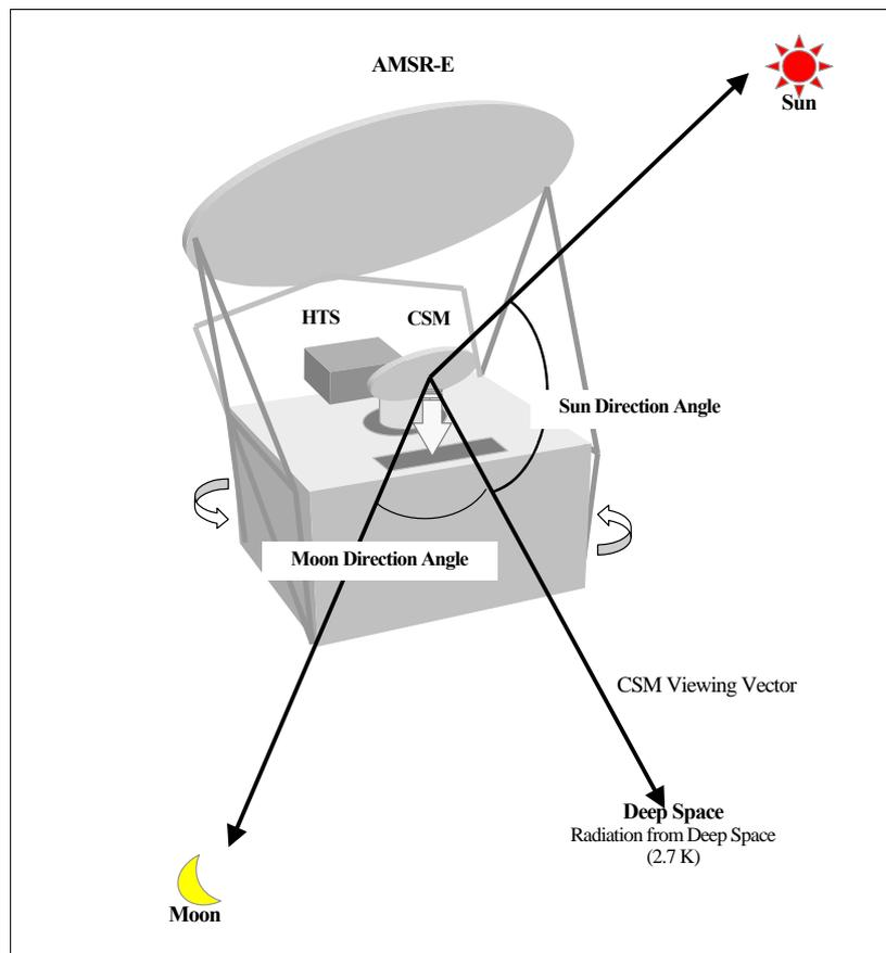
Figure 2.3-5 definition of the Moon Direction Angle and the Sun Direction Angle
