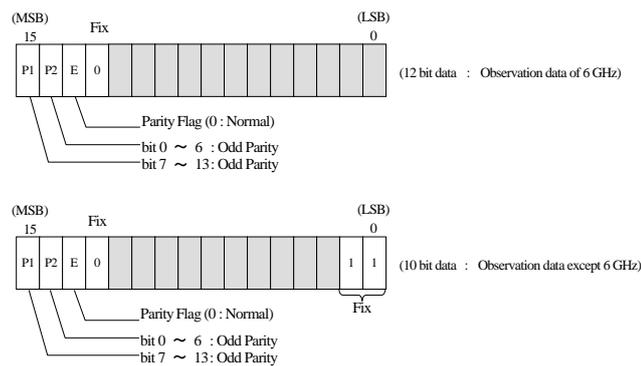
Figure 2.1-2 Bit formats of observation data (raw data)
