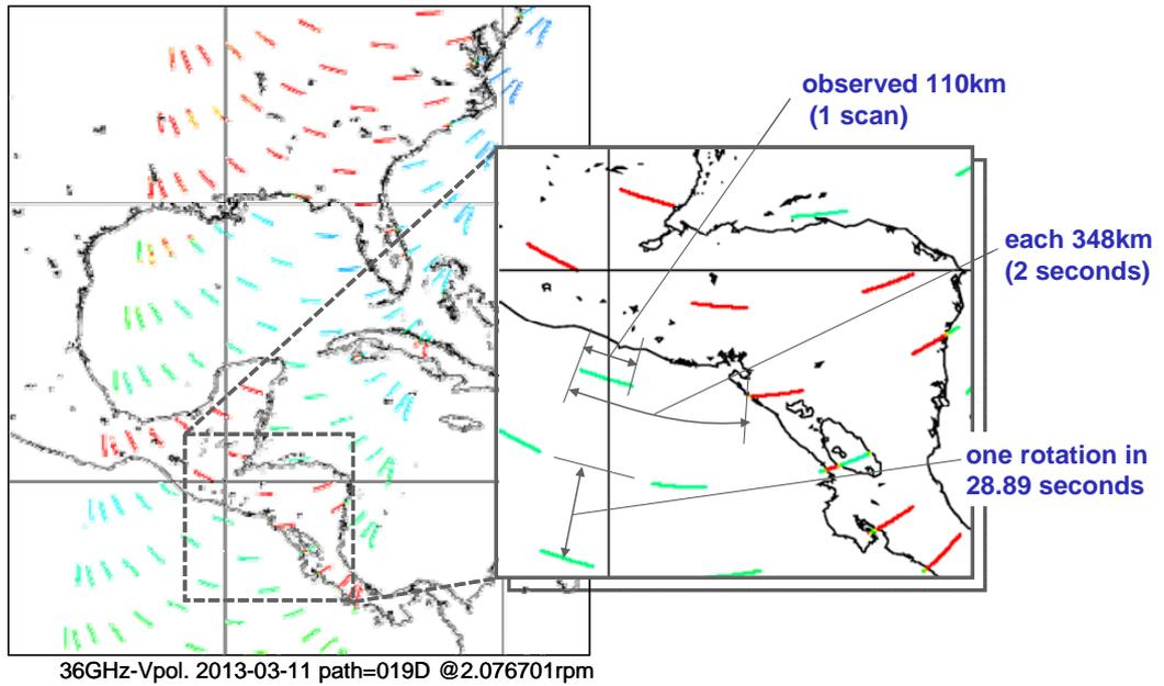
Figure 3.3-2 Schematic diagram of AMSR-E observation
