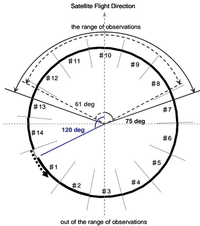
Figure 3.1-2 Geometry of the range observations of AMSR-E Slow Rotation Data
