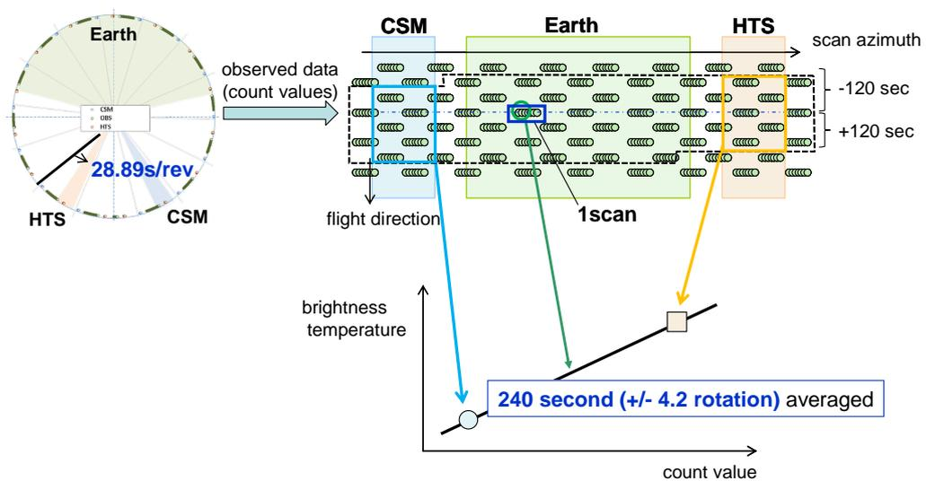
Figure 3.3-3 The range of the calibration data used for calculation of brightness temperature
