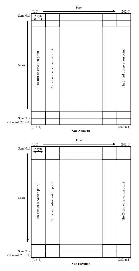
Figure 3-8 Structure of Sun Azimuth / Sun Elevation
