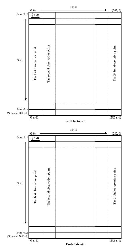
Figure 3-9 Structure of Earth Incidence / Earth Azimuth
