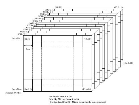
Note : The data of 6GHz-V and 6GHz-H are stored in 7GHz-V and 7GHz-H dimension, respectively.
