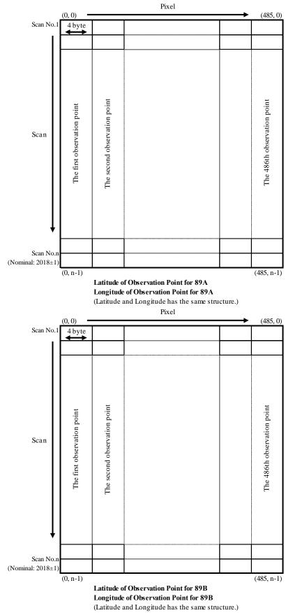
Figure 3-7 Structure of Latitude of Observation Point / Longitude of Observation Point
