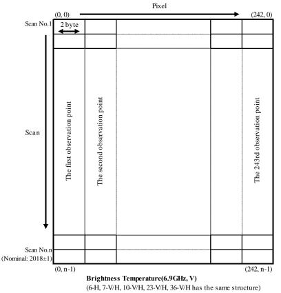
Note : Data in the 6 GHz band before bias correction is stored in 7-V/H.
