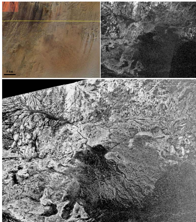
Figure 3. Landsat (top left), JERS-1 (top right) and PALSAR image (bottom) of a region located around 21°55'N, 26°36'E. PALSAR much better reveals paleodrainage channels in the lower part of the scene (JAXA/METI).
