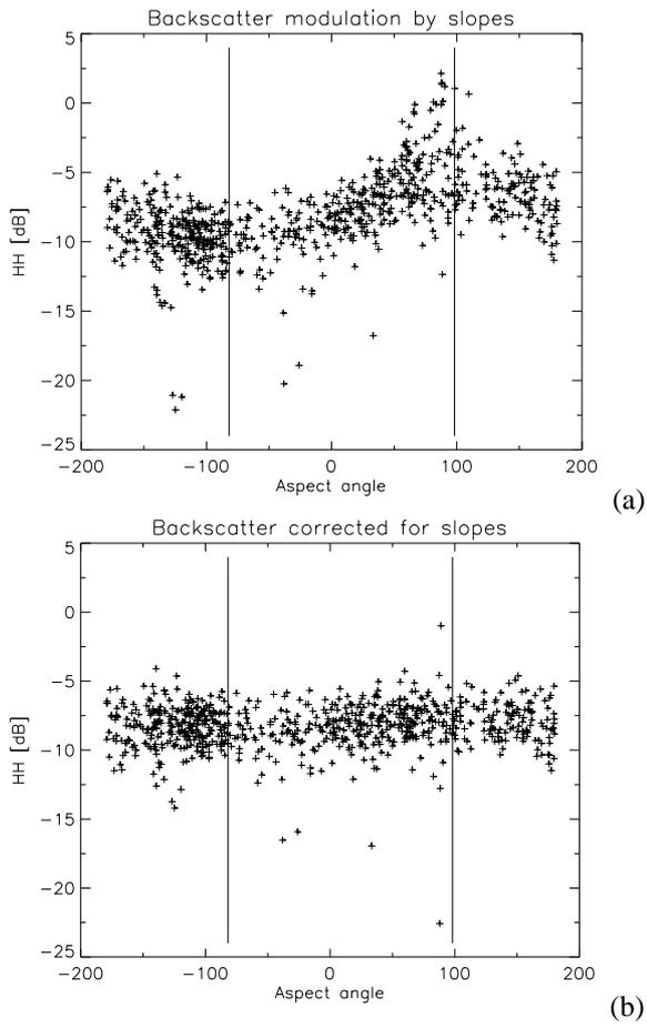
Figure 3. Slope correction for all pixels in a small test area in a mountainous section of central Borneo; (a) backscatter (gamma in dB) as function of slope aspect; (b) idem, after correction (Note: the vertical lines present the radar orientation angles).
