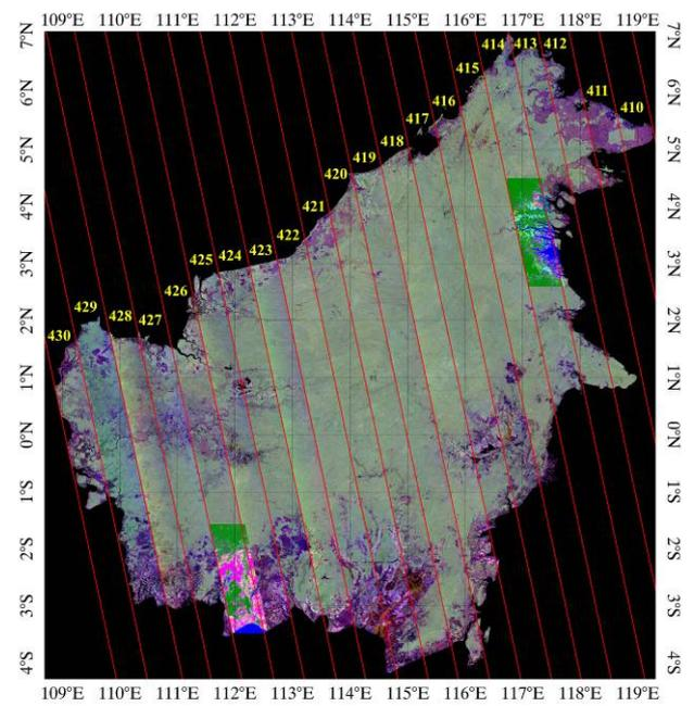
Figure 5. FBS/FBD mosaics of Borneo after radiometric balancing and slope correction. The RSP strips and two patches of classified data are superimposed. ALOS K&C © JAXA/METI
