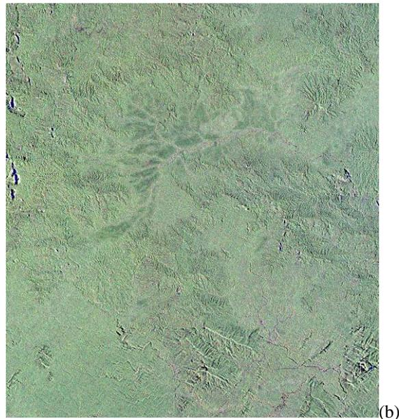
Figure 4. (a) PALSAR FBS/FBD aggregate for an area (~42x46km) typical for the mountainous forested terrain in the centre of Borneo; (b) idem, relief corrected. Some effects of overlay and shadow remain visible and are masked after classification. ALOS K&C © JAXA/METI
