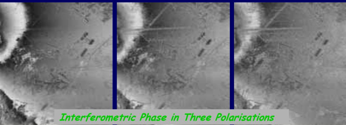
Interferometric Phase in Three Polarizations
