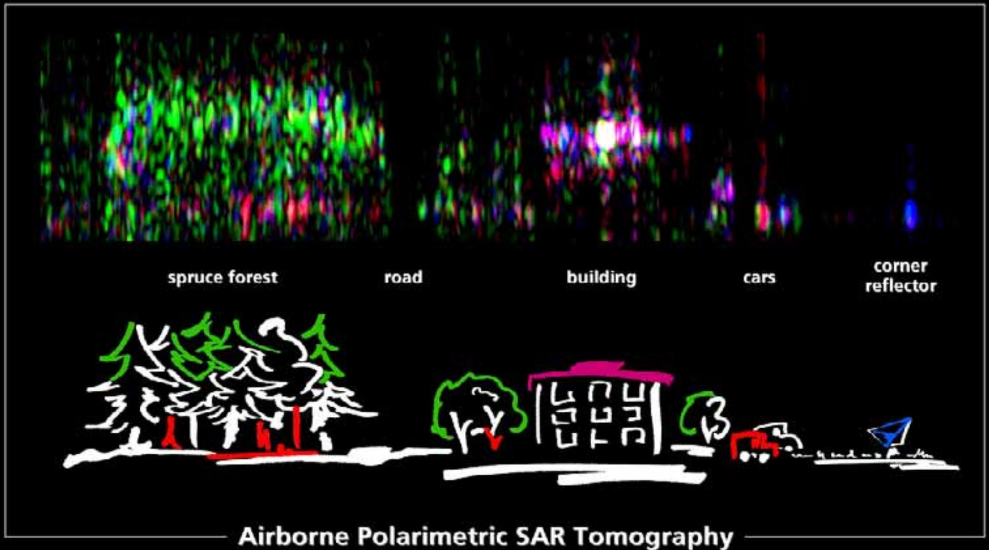
Upper image: Polarimetric color composite (L-band) of a tomographic slice in the height/azimuth-direction
