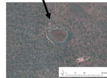
3.5m x3.5m targets were laid out and used as ground control points; positions were recorded with differential GPS
