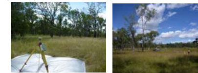
3.5m x3.5m targets were laid out and used as ground control points; positions were recorded with differential GPS
