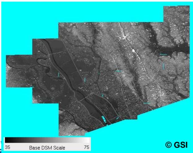
Reference Lidar/DSM by GSI.
