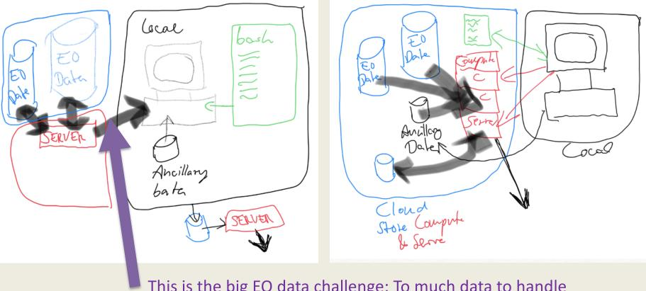
This is the big EO data challenge: To much data to handle in the era of time series high-res data sets from new SAR/optical/lidar ... missions (e.g. NISAR 100TB/day)
