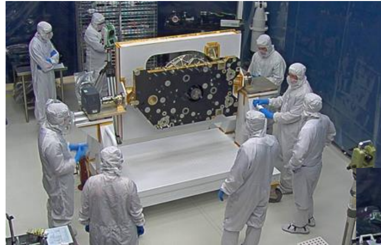
Integration of Optical Bench with Mirror Assembly
