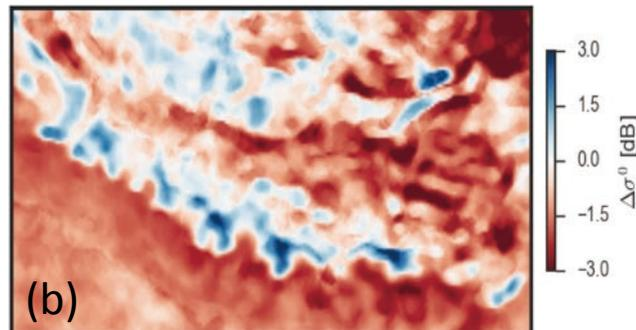
Scatterometer observations from ASCAT (A+B) characterize seasonal transitions and surface state at a regional scale (a). The enhanced resolution C-Band scatterometer product is close to 5 km. The seasonal response of ASCAT over glaciers is dictated by absorption in the snow volume and increased surface scattering over land (b).
