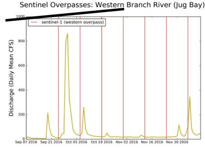
Tides vs. discharge: October 18<sup>th</sup> image is brightest presumed due to inundation underlying marsh grasses causing double bounce scattering. But it remains unclear whether tides or lagged discharge is the source of the inundation.
