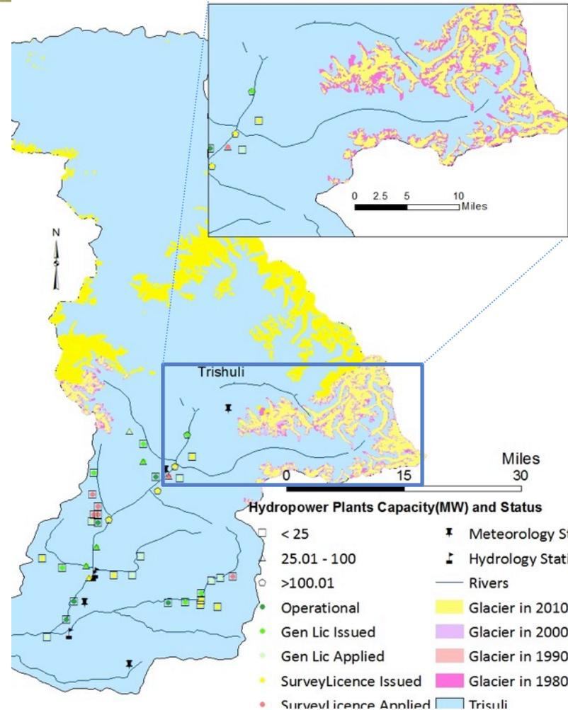
**Hydropower Plants Capacity(MW) and Status**
