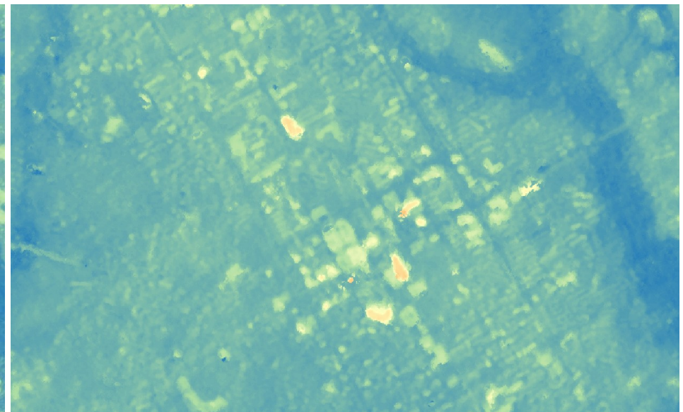
5 m-mesh DSM using ALOS PRISM.
