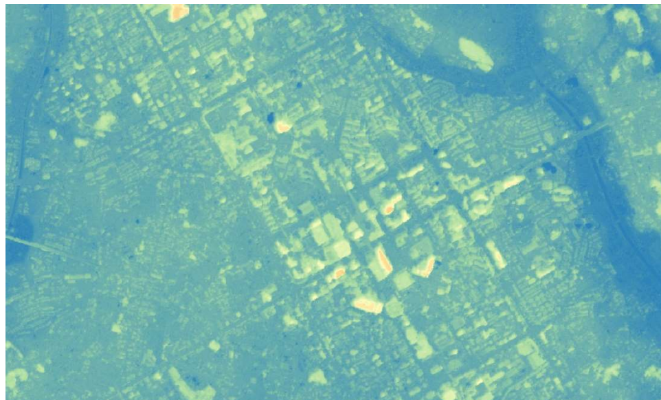
0.8 m-mesh DSM using ALOS-3 simulated image.
