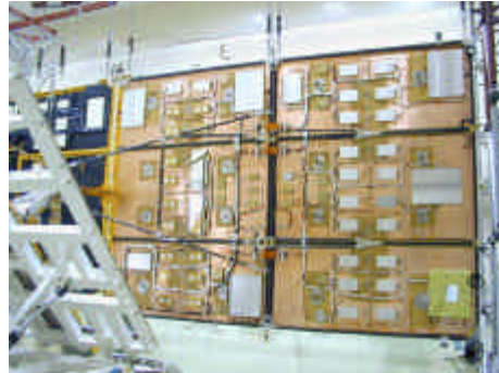
Opposite side (T/R modules and RF Dividers)
