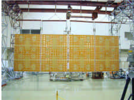
Four Antenna Panels fully deployed
