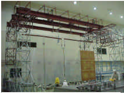
PALSAR BBM (~ Dec., 1998) Mechanical Model (Deployment, Acoustic, Separation Shock)
