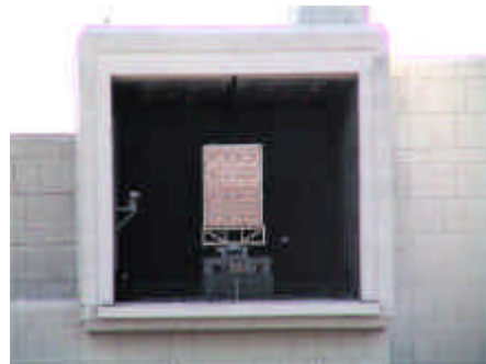
One Antenna Panel of PALSAR (Azimuth Pattern Measurement)
