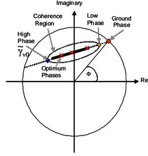
Figure (1) The schematic view of unit circle for two-layer RVOG model.
