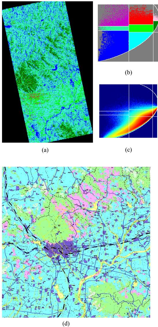
Fig. 3 Entropy-Alpha segmentation result (a), the legend for 8 terrain types (b), the occurrence histogram for each of the 8 types, and (d) is the corresponding land use map as true.
