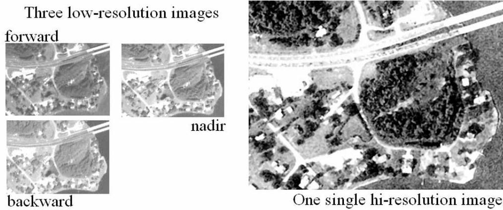
Fig. 4, A triplet of three low-resolution images (forward, nadir, and backward), and one hi-resolution image. (The hi-resolution is an airphoto, and it is not derived from the triplet.)
