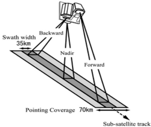
Fig. 3, Geometric configuration of individual sensors of the PRISM (from the JAXA web site).
