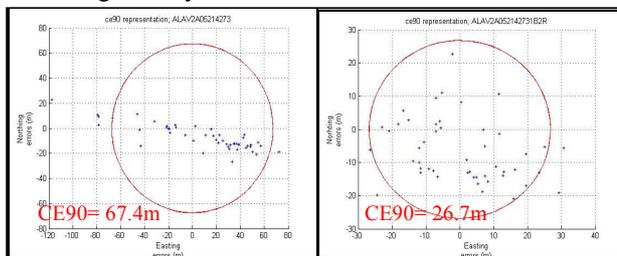
Figure 4. AVNIR-2, product geo-location (CE90), data corrected from the biases (left) and data corrected from terrain relief effect (right).
