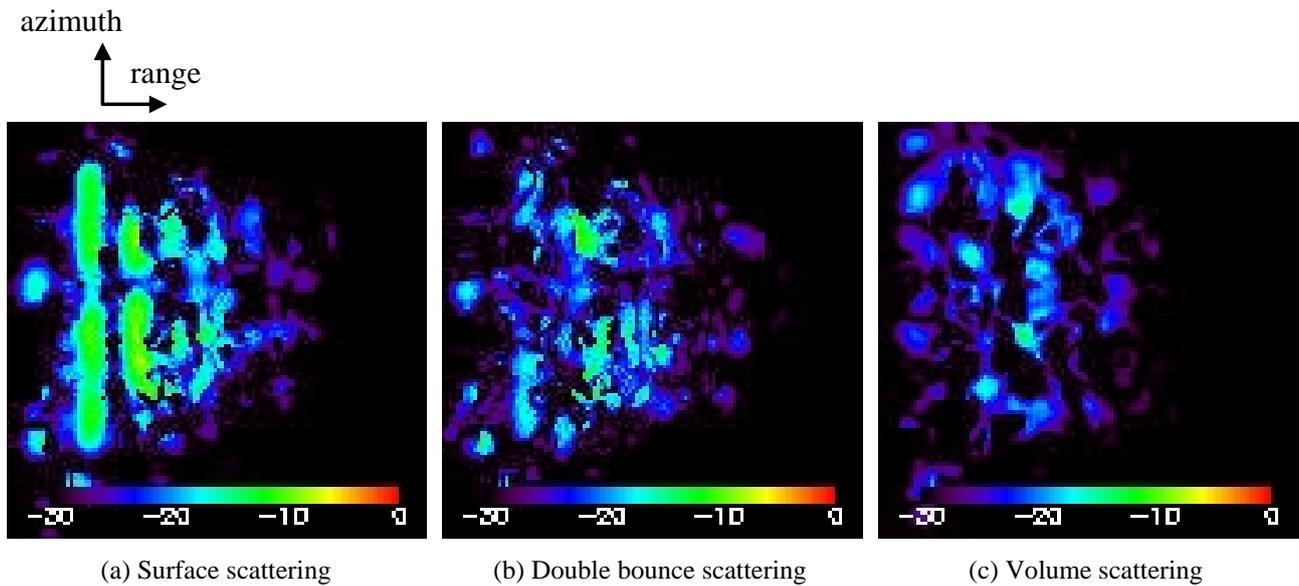
*Figure 5. X-band scattering from the specimen with 10-cm depth of water, and with paddy*
