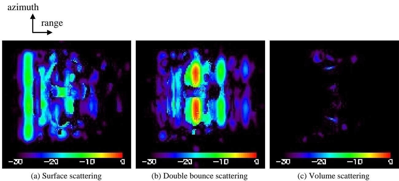
*Figure 4. X-band scattering from the specimen with 10-cm depth of water, and without paddy
