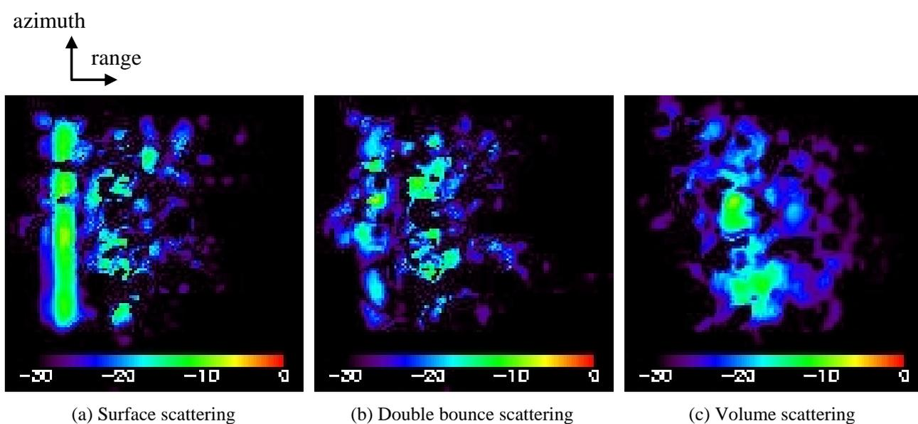
Figure 3. X-band scattering from the specimen with 1-cm depth of water, and with paddy
