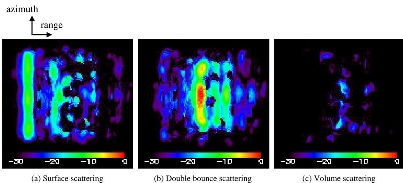
Figure 2. X-band scattering from the specimen with 1-cm depth of water, and without paddy.
