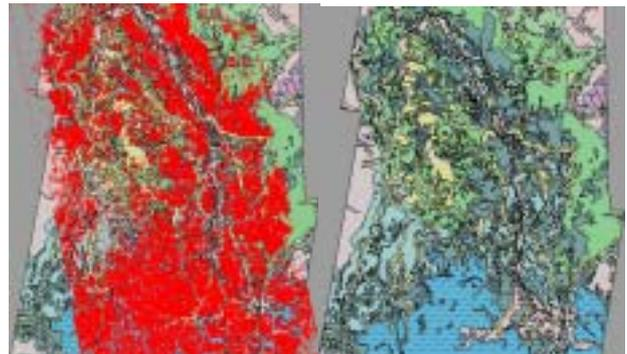
Figure 6. Geo-morphological survey map [5] (right) and the superimposed flood possible areas calculated by mathematical morphology operation from PALSAR image. (left: red color)
