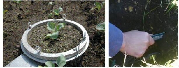
Figure 3. Lysimeter and soil moisture sensor.
