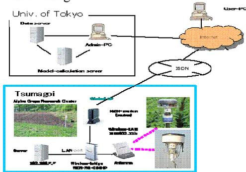
Figure 2. Field Server monitoring system.
