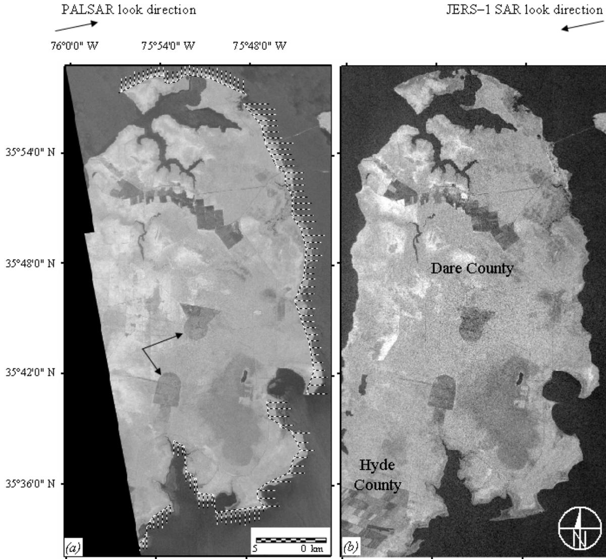
Fig. 2, (a) PALSAR HH data. Three baselines and one hundred twenty transects are shown in white-dotted lines. Two U.S. military bombing ranges are pointed by two black arrows. (b) JERS-1 L-HH SAR data. (After Wang and Allen 2007).
