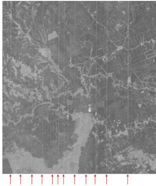
Fig. 1 Linear noise (Red arrows) in satellite direction (Azimuth)
