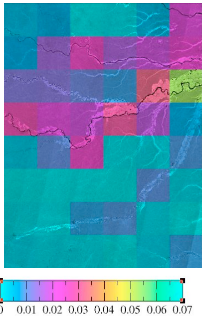
Figure 17a) Fractional open water May-June 2007, tile 19M. The fraction of open water varies from 0 (green) to 5 %. (yellow)
