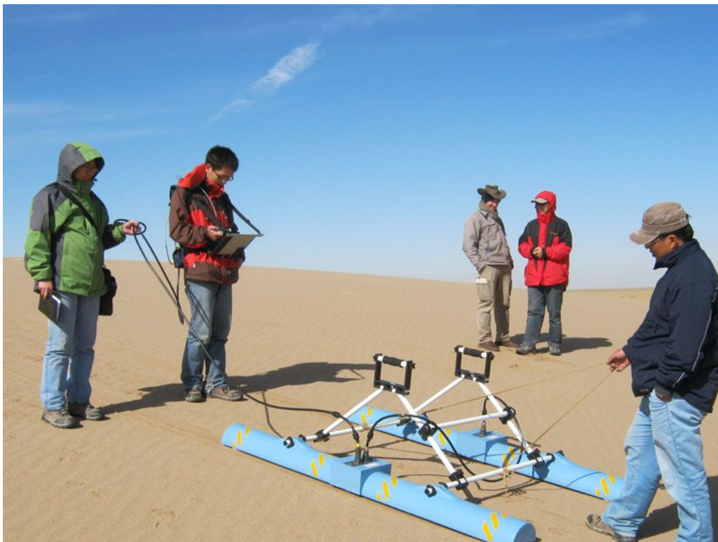
Figure 6. Top: Lacustrine sediment outcrop that was localized with the help of SRTM and PALSAR data. Bottom: Ground Penetrating Radar sounding of a recent sand dune in the Hunshandake desert.
