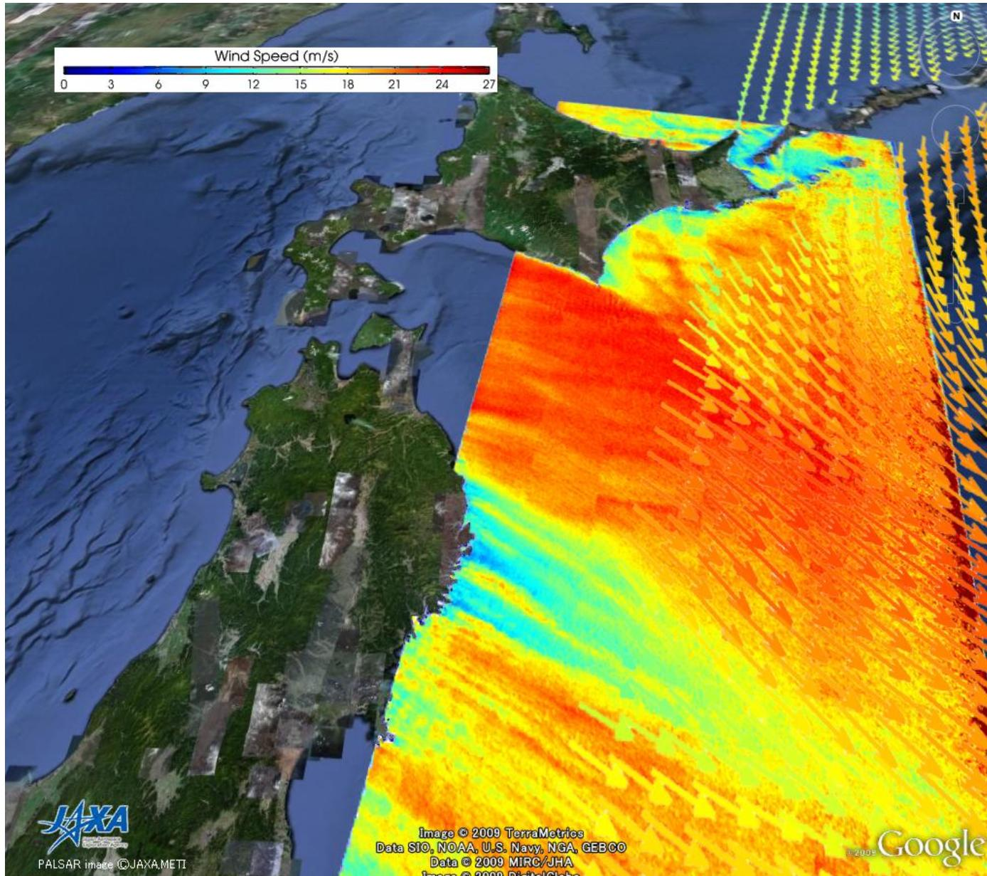
Wind Speed Measurement Using the PALSAR/ScanSAR
