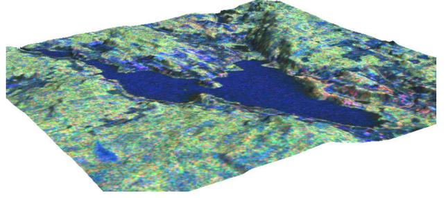
Figure 1. Polarimetric view of Kuortane 2007-05-14. Red = HH-VV, green = HV, blue = HH+VV. ©JAXA and METI 2007.
