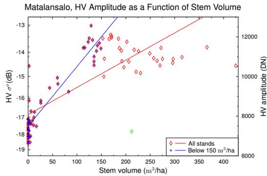
Figure 4. HV amplitude of Palsar/Dual-polarized data as a function of forest stem volume. Heinavesi site, 2007-06-12.
