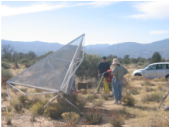
Figure 2. Photographs of one of the 3 radar reflectors. Reflectors D1 and D2 were installed at Pinon in 1997 were originally oriented to reflect radar from ERS-1 and ERS-2 having incidence angles of 23° and azimuth of 102.5°. In July of 2004 the reflectors D1 and D2 were adjusted to optimally reflect ALOS data with incidence angles between 34° and 43°. In November of 2005 the ascending reflector was installed to reflect radar waves having an azimuth of 257.5° to reflect ALOS data along ascending passes.
