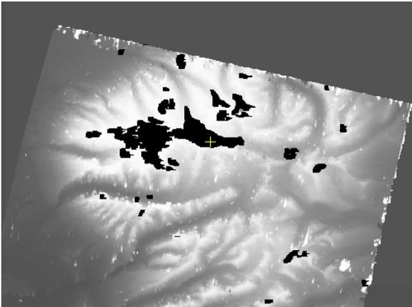
Figure 7. The generated DEM from ALOS/PRISM 1B2
