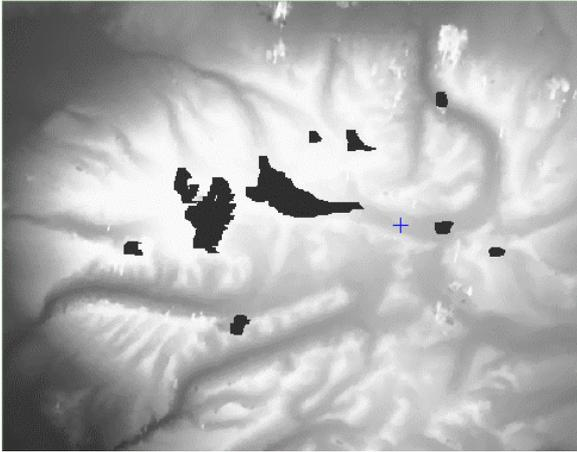
Figure 6. The generated DEM from ALOS/PRISM 1A
