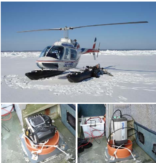
Figure 1. Photos were taken either with a Nikon D200 digital camera (bottom left) or a FLIR A40M infrared camera (bottom right) through a hole in the hull of the helicopter. Photos: Henrik Lindh, Leif Eriksson.
