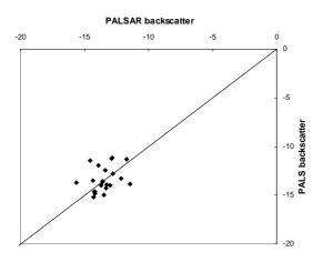
Figure 3. Comparison of PALSAR and PALS HH polarization radar backscatter for intensive soil moisture sampling sites in the Little Washita watershed on July 1, 2007. Each field is 800 m x 800 m.
