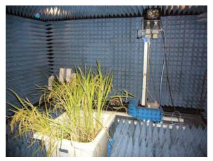
Figure 1. Measurement of specimen using fully polarimetric FM-CW SAR system with X-band, developed by Yamaguchi et al. [4]
