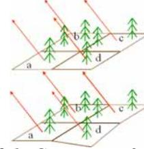
Figure 2.1 Geometry of four-pixel blocks for land surface monitoring: undisturbed (upper) or with a small disturbance in block d (lower).
