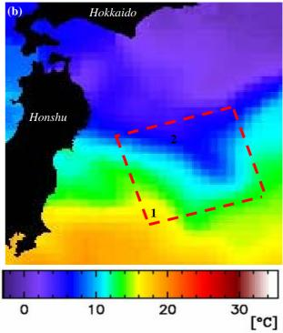
Figure 4. (a) ALOS PALSAR image acquired on 18 April 2006 and (b) New Generation Sea Surface Temperature map produced at the same day by the Tohoku University http://www.ocean.caos.tohoku.ac.jp/~merge/sstbinary/ showing correlation between radar and thermal contrasts.
