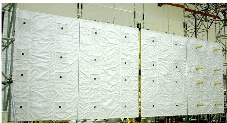
Fig. 4. PALSAR antenna during deployment tests.
