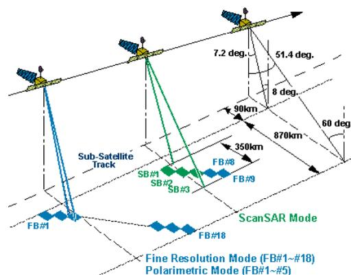
Fig. 5. PALSAR observation characteristics.
