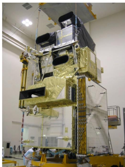
Fig. 2. ALOS Prototype Flight Model, nadir facing the camera.
